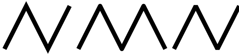
Figure 4: The meaning of the option linejoin=0|1|2 for drawing lines
